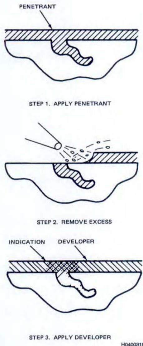
Figure 2-1. The Penetrant Inspection Process
