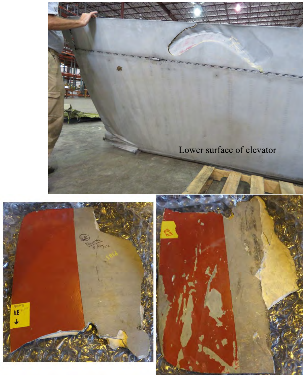
Figure 45: Lower Surface of Elevator near HSS 95 – HSS 130 Blade tip fragment from Propeller #3, Blade 3
