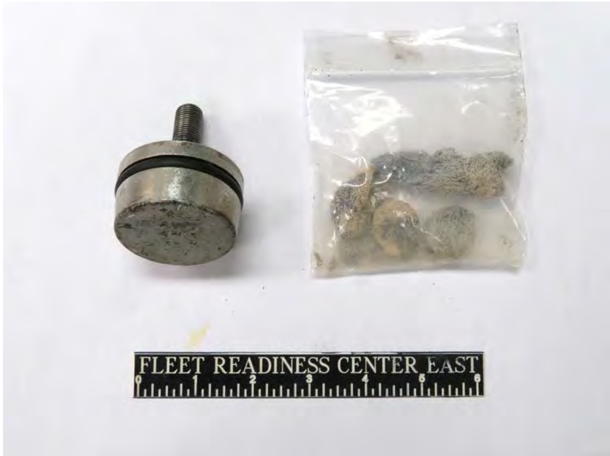
Figure 11 - Taper bore plug and lead wool showing corrosion damage
