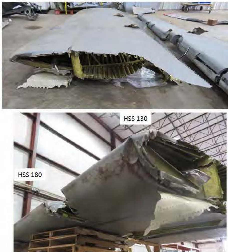
Figure 34: HSS 130 Impact Damage Leading Edge of Horizontal Stabilizer RH outer section
