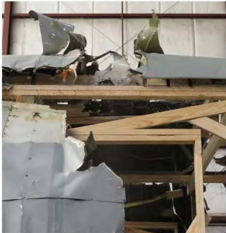
Figure 11: Blade 4 of Propeller #3 Impact Site on LH side of Center Fuselage
