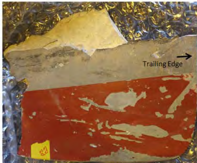
Figure 46: Propeller #3, Blade 3 Damage likely caused by intrusion into center fuselage airframe structure
