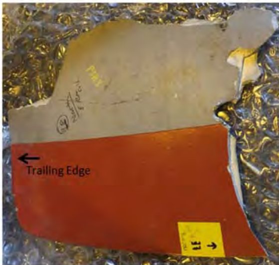
Figure 46: Propeller #3, Blade 3 Damage likely caused by intrusion into center fuselage airframe structure
