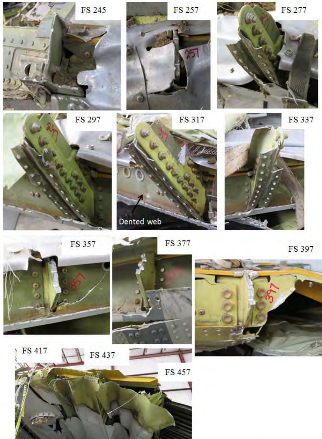
Figure 28: Left Side Floor Fitting to Ring Segment Joint along Chine Assembly
