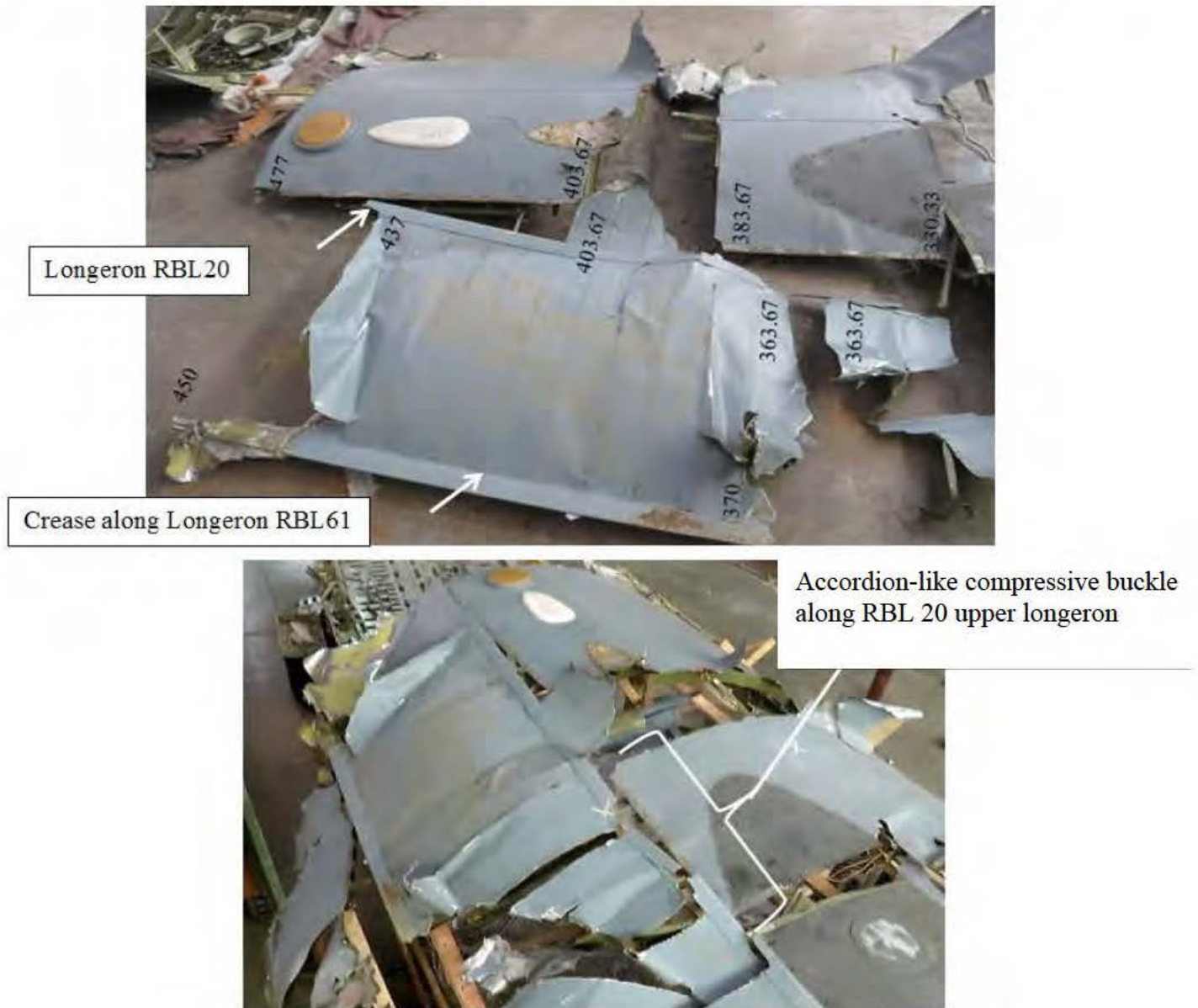
Figure 20: Closer view of Fuselage Center Section Upper Surface STA 330-477
