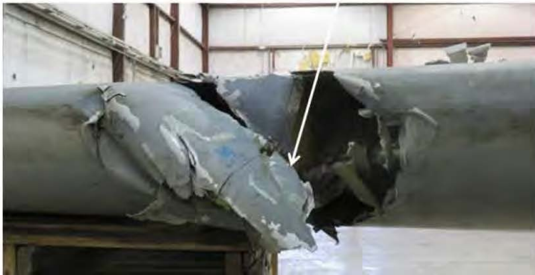
Figure 36: HSS 180 Impact Damage Leading Edge of Horizontal Stabilizer RH Outer Section
