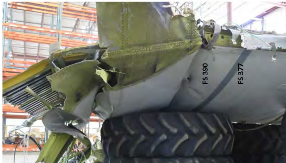
Figure 31: Right Side Floor Fitting separation aft of FS 390
