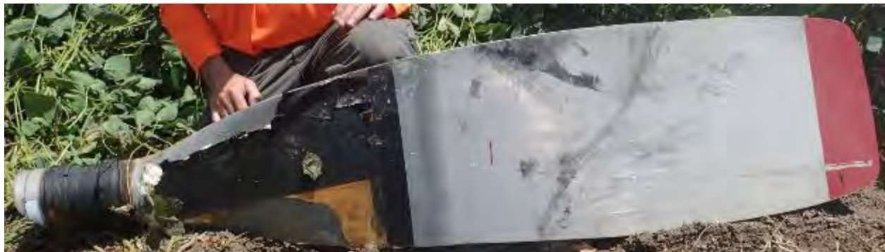
Photograph 3. North Debris Propeller Blade From #2 Engine
