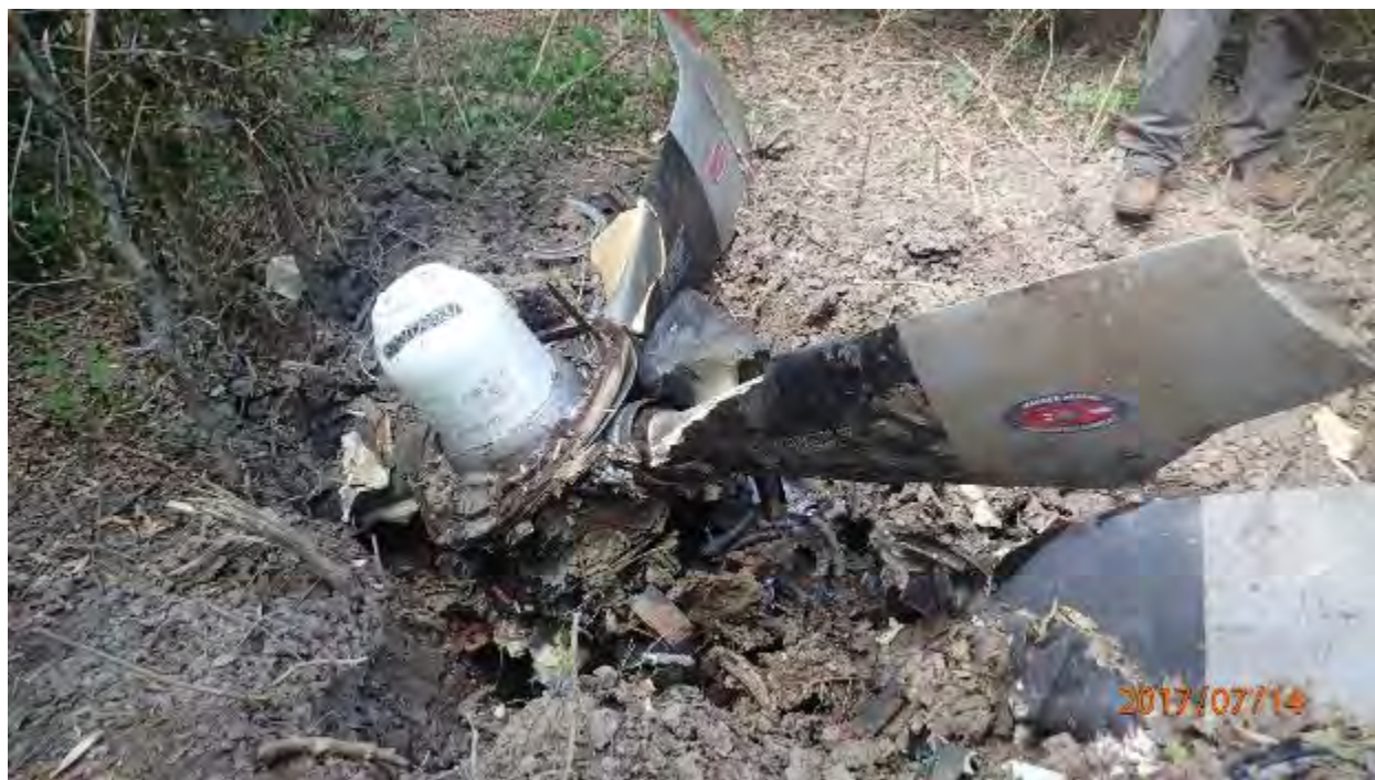
Photograph 6. North Debris Field Propeller Blades, Hub and Rotary Gear Box From #3 Engine, Blade Angles Approximately 90 Degrees
