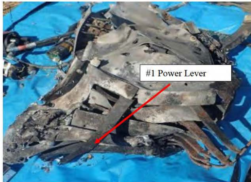
Photograph 15. North Debris Field Power & Condition Levers
