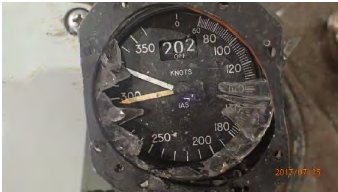
Photograph 17. North Debris Field Airspeed Indicator #1
