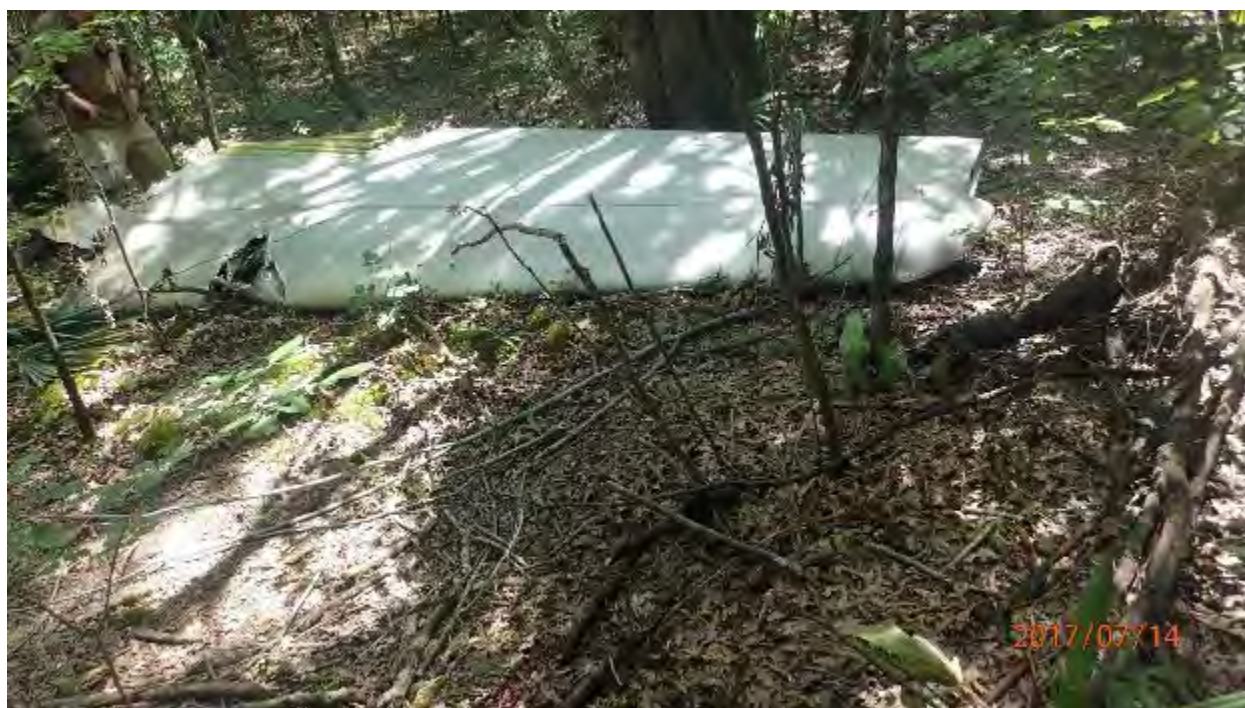
Photograph 7. North Debris Field Portion of Right Horizontal Tail
