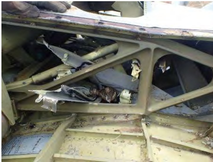
Photograph 10. Rudder Actuation Fitting
