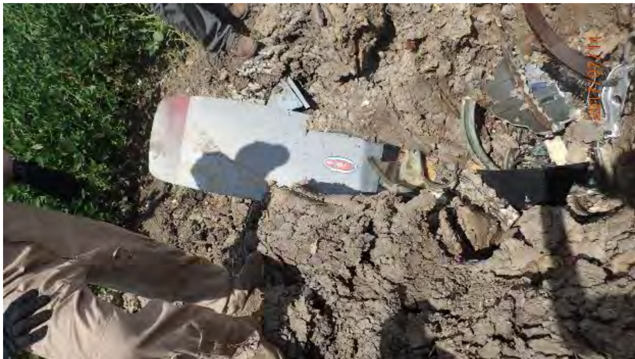
Photograph 4. North Debris Field Rotary Gear Box and Propeller Blades from #2 Engine
