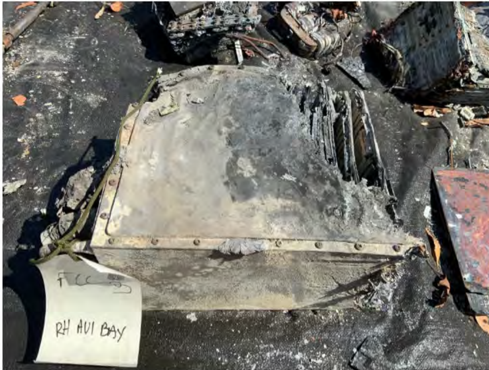
Flight Control Computer as recovered in the field
