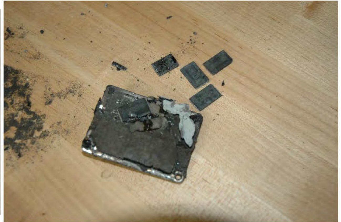
Delaminated memory chips and damaged circuit card
