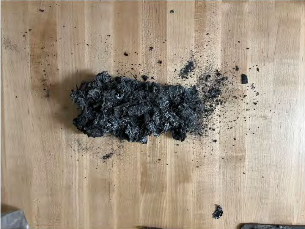
Melted asset with visible circuit card
