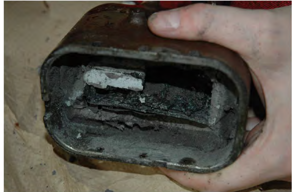
Exposed circuit card after initial fire resistant potting removal
