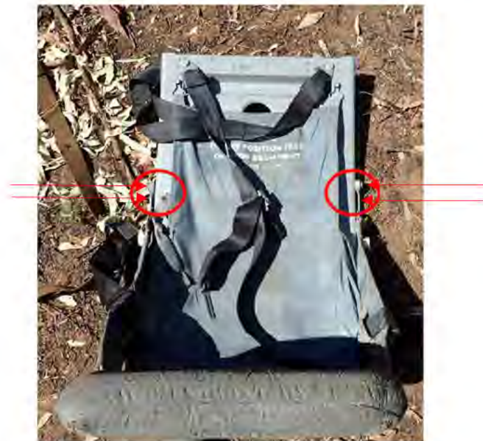
Figure 9. Photograph of detached troop seat found outside the aircraft taken from the MIST Report with red circles added to identify seat stroking. The misalignment of the faint red lines encircled in red indicates the amount the seat stroked.
