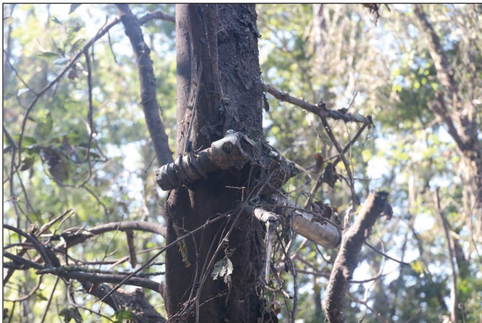
Photograph 2. Nose Landing Gear (NLG) Strut embedded approximately eight feet up tree trunk
