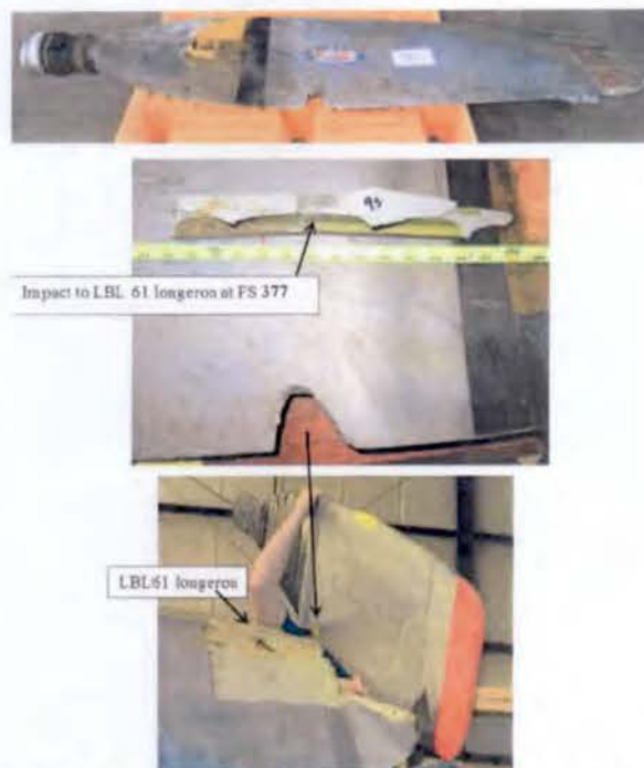
Figure 6: Reconstruction of P2B4 Impacting Port Side Panel
