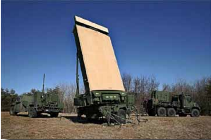
The Ground/Air Task Oriented Radar (G/ATOR) replaces five legacy radar systems and supports air surveillance, fire-finding, and air traffic control missions.
