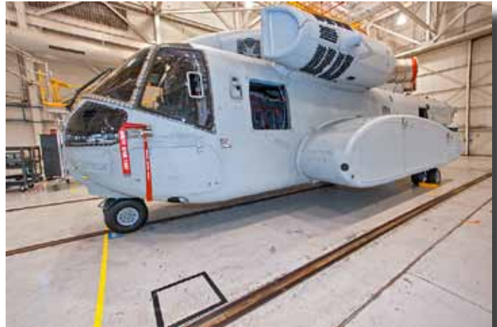
The CH-53K Ground Test Vehicle at Sikorsky’s Florida assembly and flight operations center.
