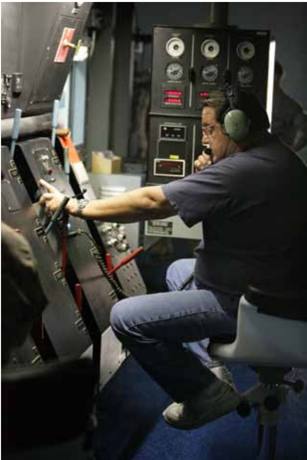
An engineer monitors & adjusts pressure levels in a chamber simulating flight in an unpressurized aircraft at Marine Corps Air Station Miramar, California.
